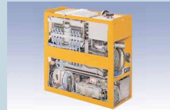
The blowers and fans in the electric system were redesigned by ebm-papst for this task: the tried-and-tested basic motors had to be reworked to ensure maximum efficiency at the required operating point of the cell. To achieve this, the motor coil and motor electronics have been specially tuned to each other.
